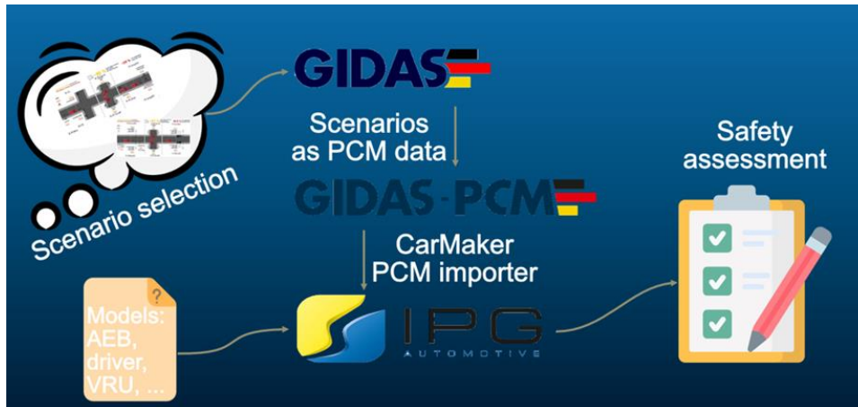
Figure 5: Process for re-simulation of GIDAS-PCM accidents in IPG CarMaker.
