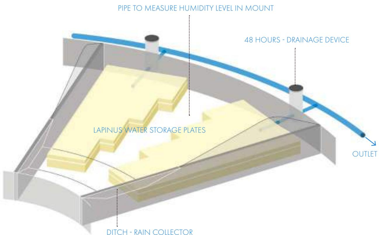
Scheme detail of the design for hydrological monitoring in the Waving wadi
