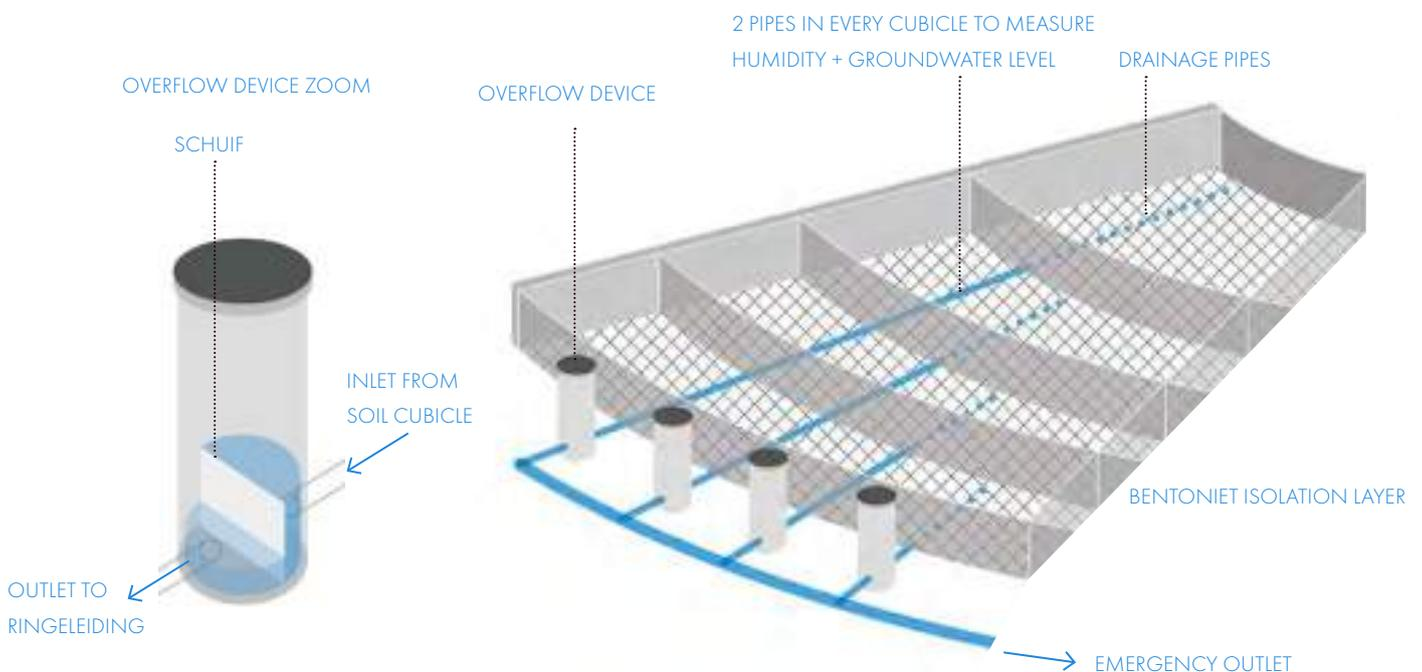
Scheme detail of the design for hydrological monitoring in the Soil cubicles.
