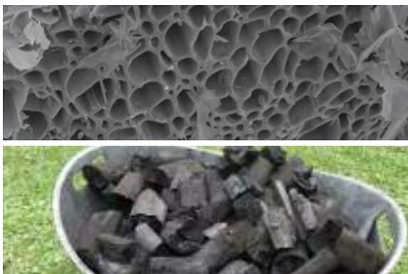
*Biochar is a type of charcoal used in agriculture with some added benefits: it has potential to help mitigate climate change effects by capturing carbon; it has the ability to attract and retain water; and it has the ability to improve soil fertility of acidic soils and to increase agricultural productivity.*
