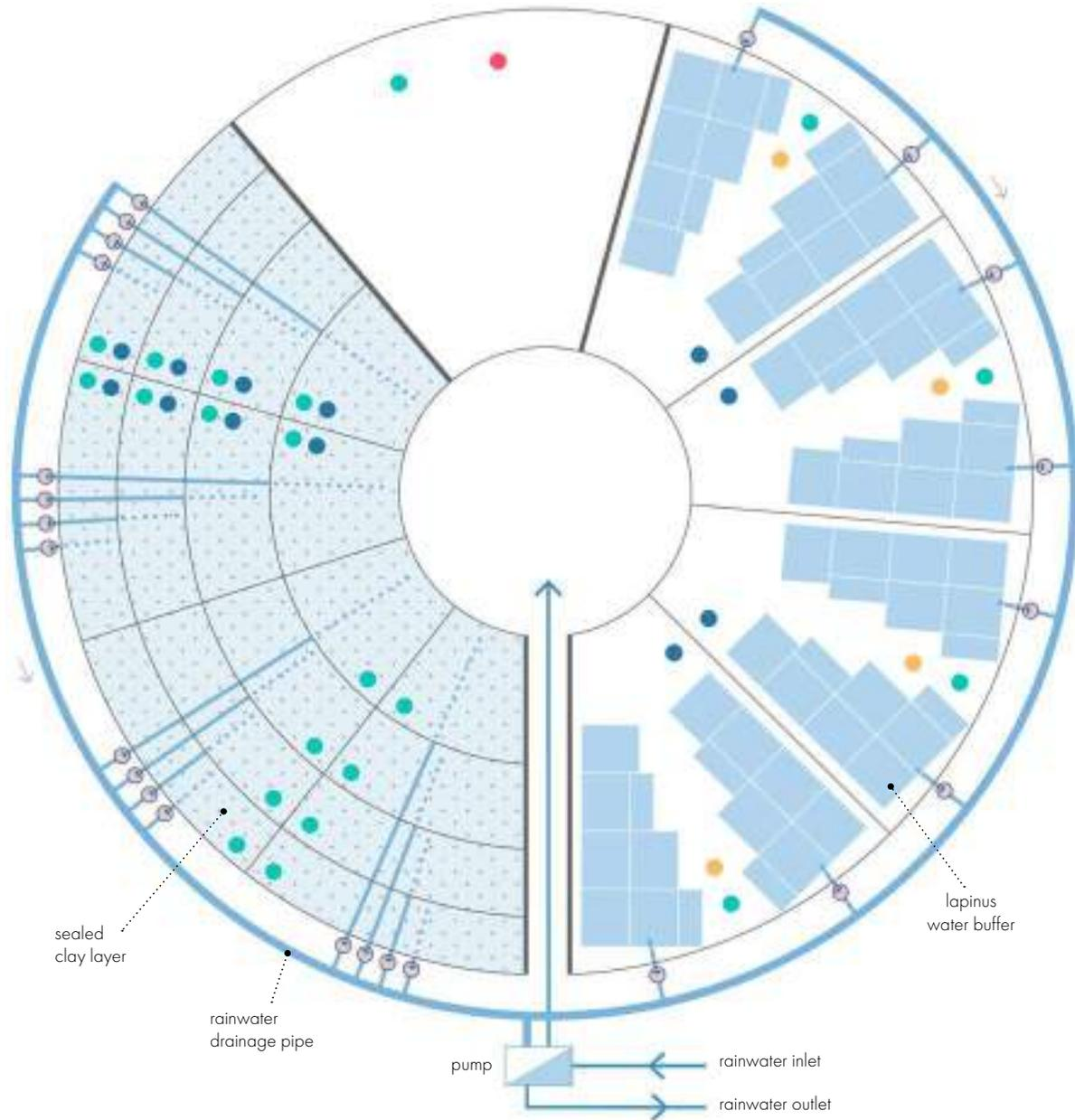
Setup of the hydrological monitoring infrastructure of the test-site
