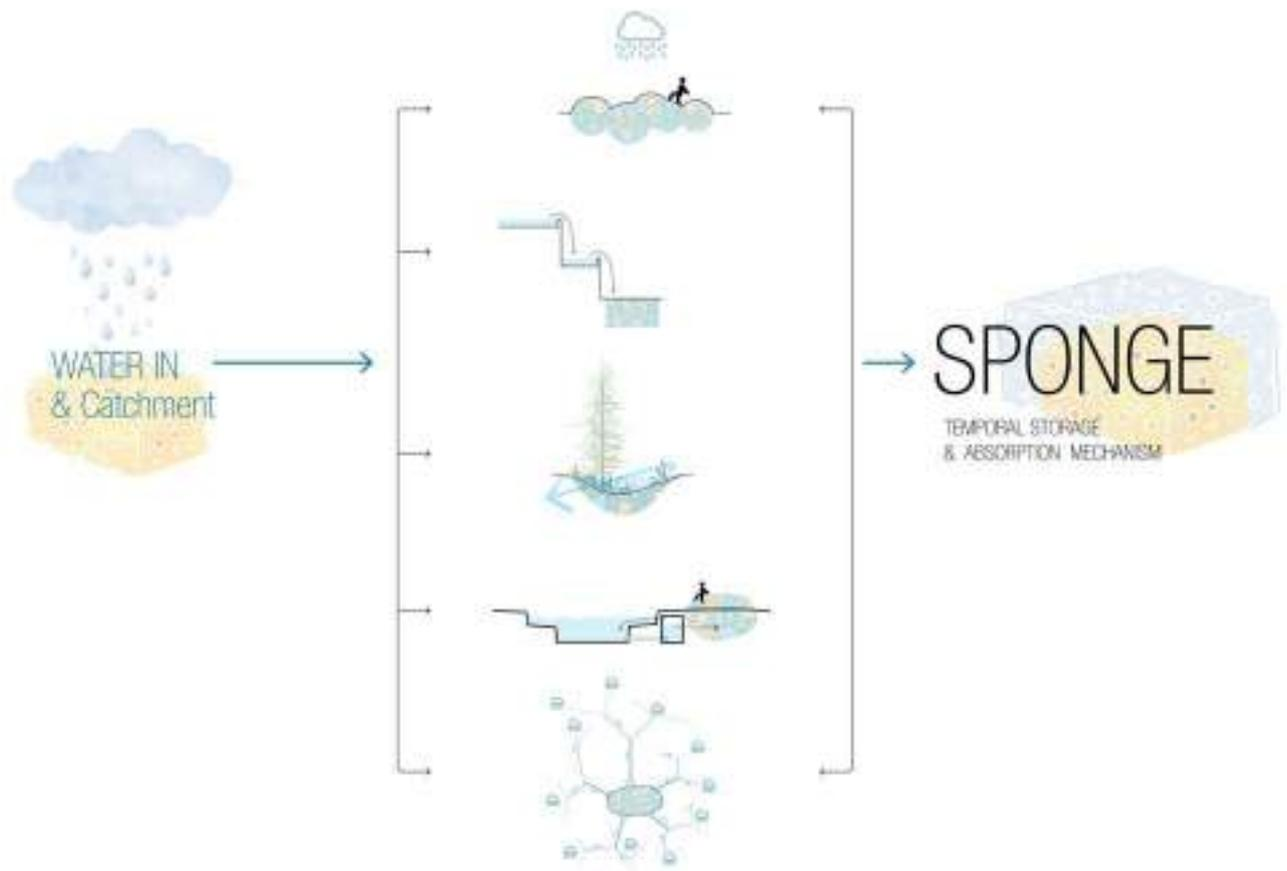
The mechanism of how a sponge can work, follows a threefold sequence of collecting water, storing it for a certain period and then returning the water into the ecosystem. This 'Collect - Store - Return' sequence implies that the concept of a sponge is in essence a system.
