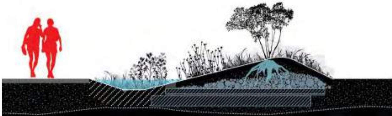
Schematic setup of the waving wadi
