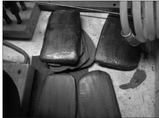
Figure 3. Replica plaques in various stages of production: plaque 'rough-outs' being ground into shape (left); polished plaque 'blanks' ready for engraving (right).
