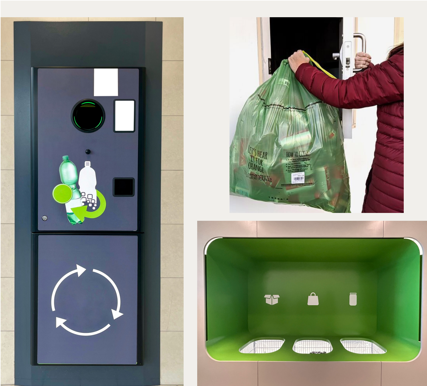
Leveraging existing DRS infrastructure for reuse systems: a reverse vending machine that accepts reusable packaging (L), a bag drop program for bottle return collecting reusables (top R), a bottle depot with a set-aside place for reusables of all shapes & sizes (bottom R).
