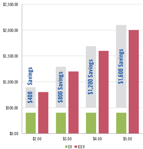
Figure B: Annual Fuel Costs to Power an EV vs. 30 MPG ICEV at Varying Gasoline Prices (assume 12,000 miles/year) 23
