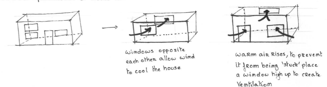
Figure 5 Sketch illustration of cross ventilation by window placement.
