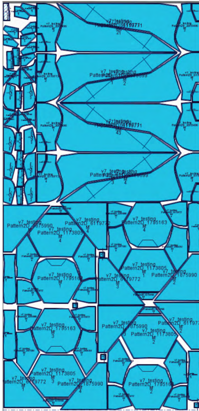
Fig. 34: Best prototype pre-factory, utilising sliding hexagon method and nesting as squares: 87%
