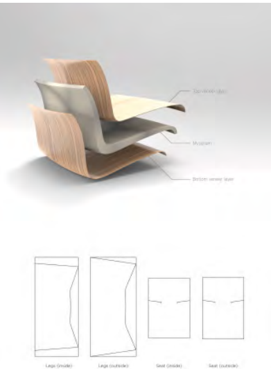
Fig. 9: Pare Chair construction and pattern detail by Glenn Catchpool ©Glenn Catchpool
