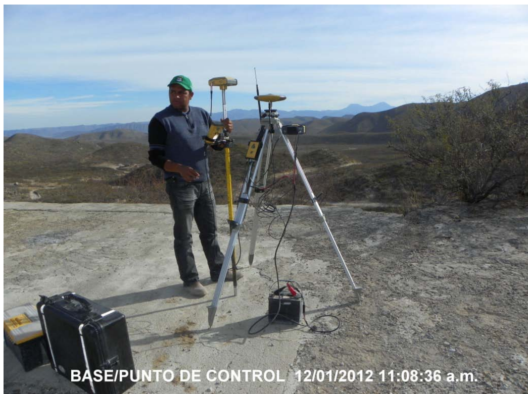
Figure 21: Base station used for the DGPS system (Galindo Surveyors).
