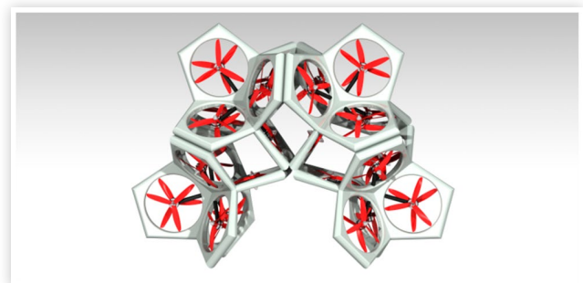
FIGURE 19 Four Lynchpin aircraft forming a flying gripper.
