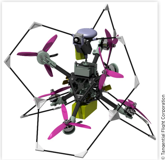
FIGURE 3 CAD model of the prototype Lynchpin.
