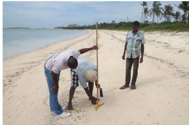
Figure 3. Measuring beach profiles (Photo: Sea Sense).
