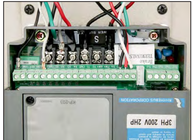
Figure 64. Inverter/Controller box wiring (see wiring diagram on Page 49 ).
