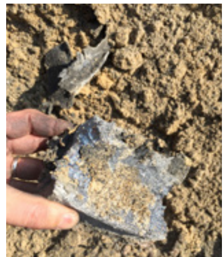
Cutting Steel: NX5600 charge used, 65mm severed
