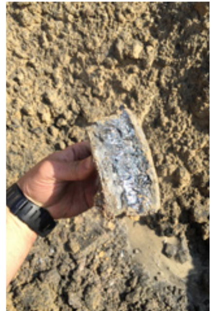
Cutting Steel: NX3600 charge used, 45mm severed
