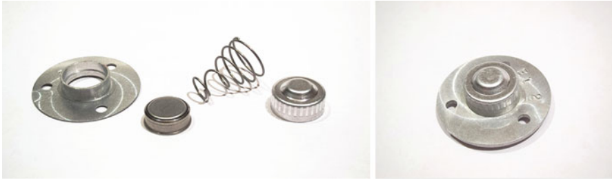
Fig. 15.7 Custom iButton case. The iButton data logger itself is the object that looks like a coin cell battery, second from the left
