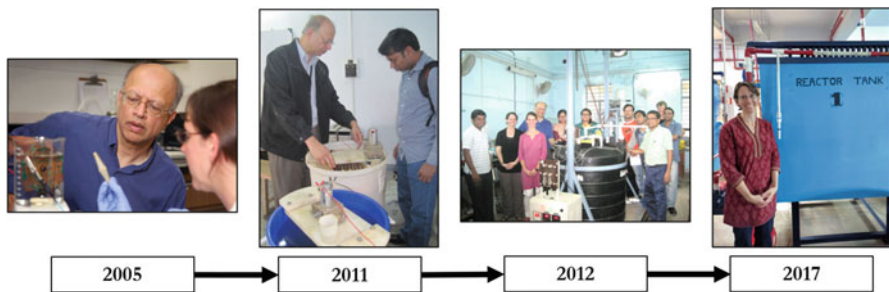
Fig. 14.4 The progression of ECAR, beginning as a 200 mL beaker, with its development to 100 L and 600 L prototypes, and finally scaled as two ECAR reactors of 1000 L each. The 2005 photo shows Ashok Gadgil and Susan Amrose at the Berkeley Lab. The 2011 photo shows Ashok Gadgil and Siva Bandaru inspecting the 100 L prototype at Amirabad High School. The 2012 photo shows Siva Rama Satyam Bandaru, Susan Amrose, Caroline Delaire, Ashok Gadgil, Paramitha Chaudhuri, Sudipta Ghosh, Suman Chakraborty, Chandan Bose, Amit Dutta, Peter Kuin, and Sayantan Sarkar with the 600 L prototype at Jadavpur University. The 2017 photo shows Susan Amrose standing next to one of the two reactor tanks at Dhaphdapi High School
