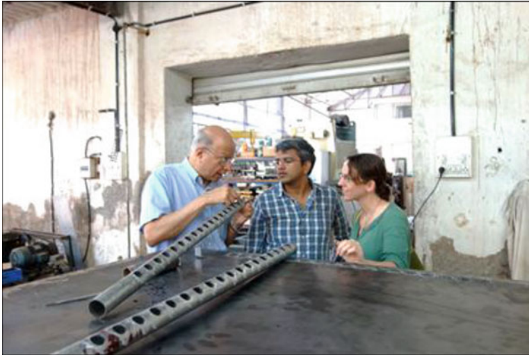
Fig. 14.3 Ashok Gadgil, Narendra Shenoy (chief design engineer of Shri Hari Industries), and Susan Amrose in November 2014, discussing the design details of the water distribution manifold for the two ECAR reactors then under construction
