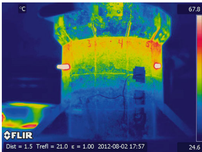
Fig. 15.10 A Berkeley-Darfur Stove imaged by an infrared camera to determine optimal iButton SUMS placement, August 2012
