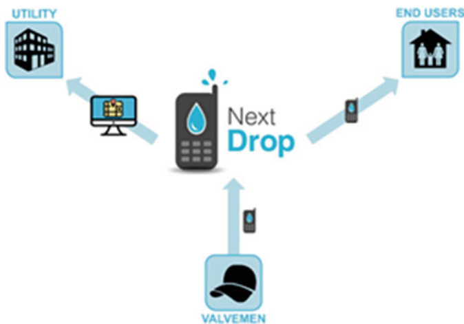
Fig. 17.1 NextDrop’s phone-based water supply notification system depended on notifications from water valvemmen. (Adapted from NextDrop)
