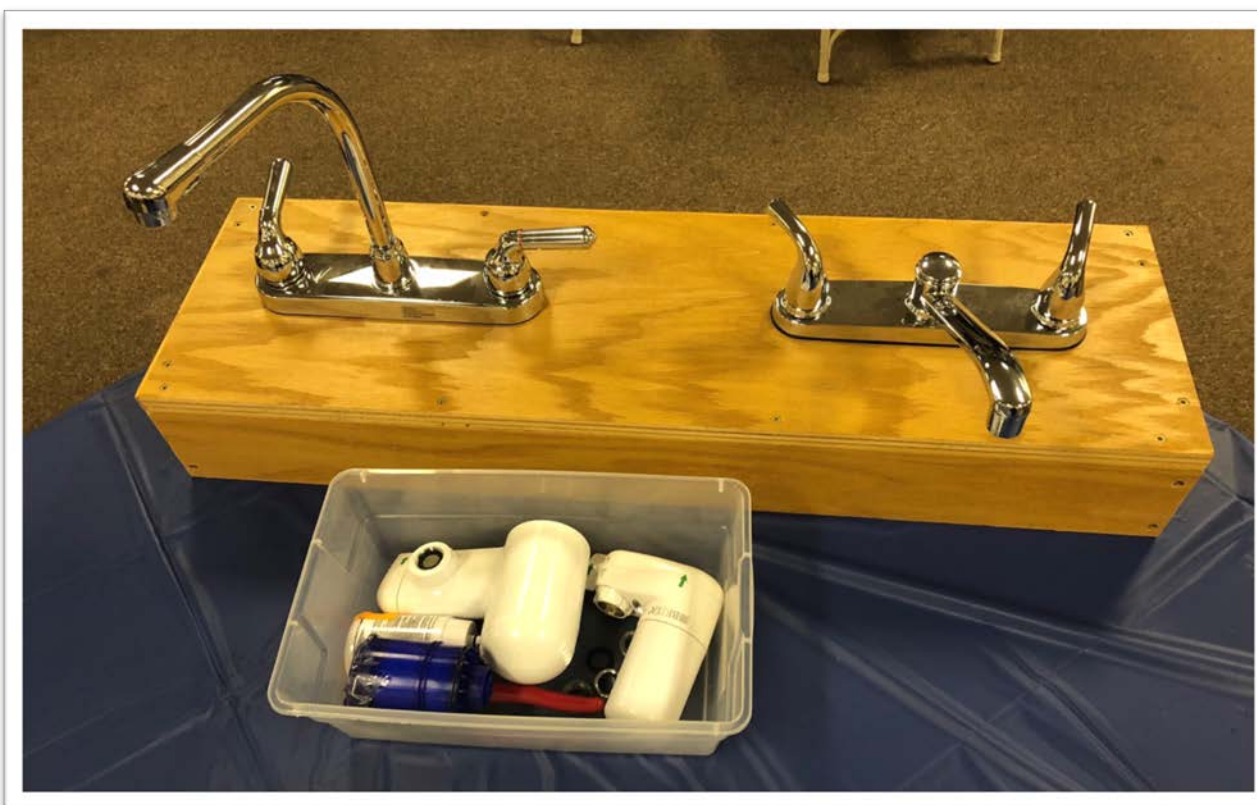
Image 4: Dry-block faucet box set up Clear box contains assembly materials (page A-4)
