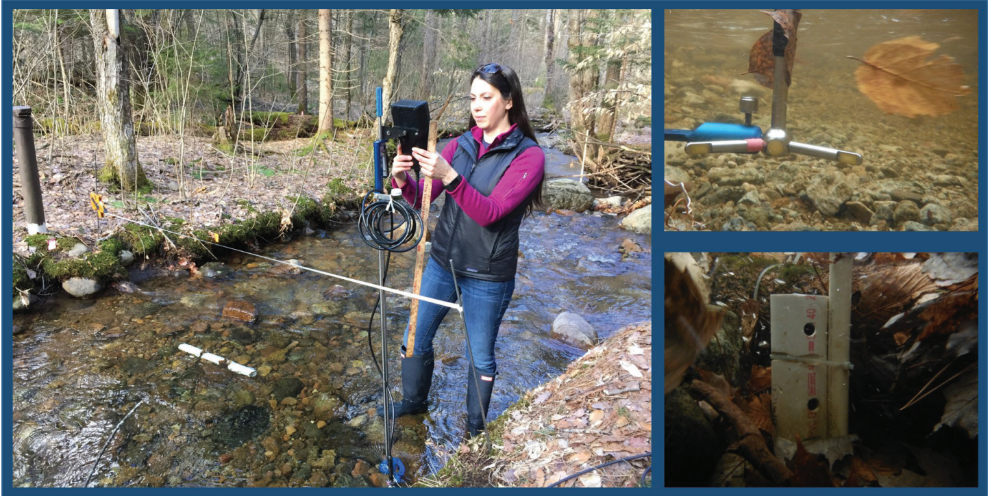
Collecting data from the Blue Mountain Lake watershed. Clockwise from left: AWI Research Associate Elizabeth Yerger quantifying stream discharge with the Flow Tracker ADV. Underwater view of the acoustic Doppler sensor of the flow tracker. Underwater view of the PVC housing that contains the Hobo conductivity meter.
