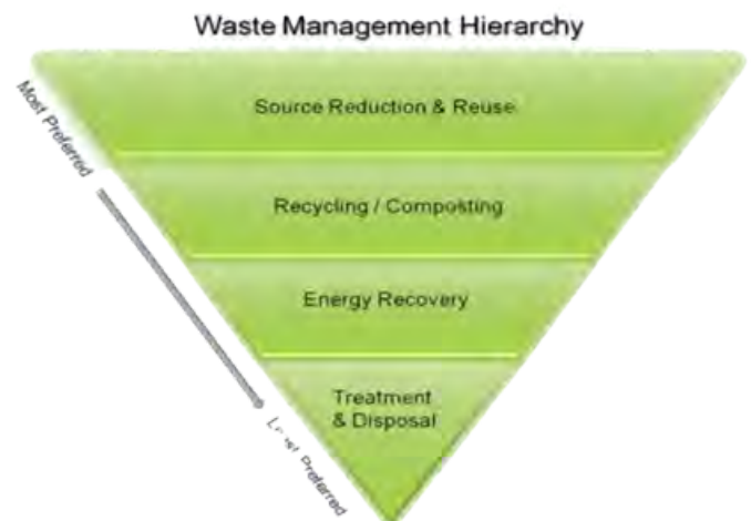
Figure 17: EPA's Waste Management Hierarchy, 2023. The hierarchy ranks the various waste management options from most environmentally preferred to least preferred. At the time this report was published, the hierarchy was under review by the EPA to see if changes should be made based on the latest available data.
