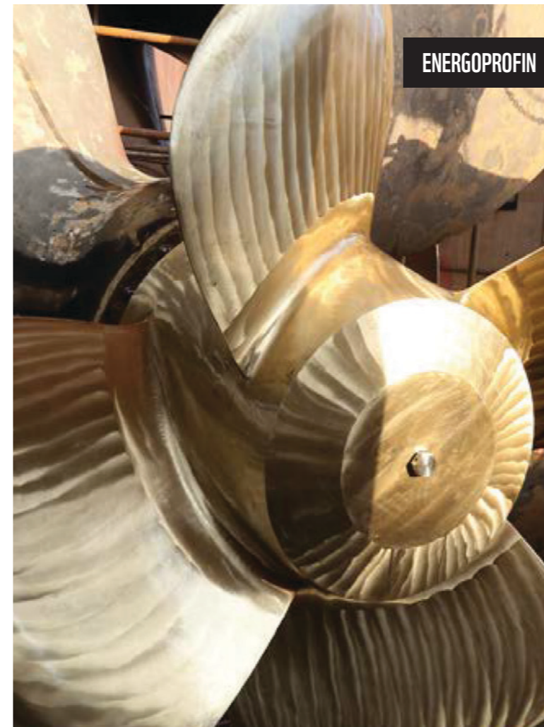
Figure 12: Illustrations of propeller designs and modifications that can reduce underwater noise from cavitation. Source: AQUO, Comprehensive listing of possible improvement solutions and mitigation measures, Deliverable D5.1, European Commission, 2014.
