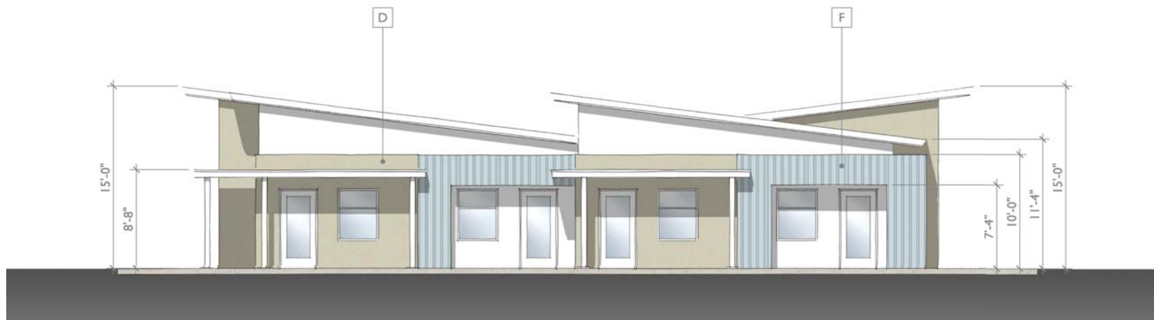
WEST ELEVATION (ROOF TYPE A') ② SCALE: 3/16" = 1'-0"
