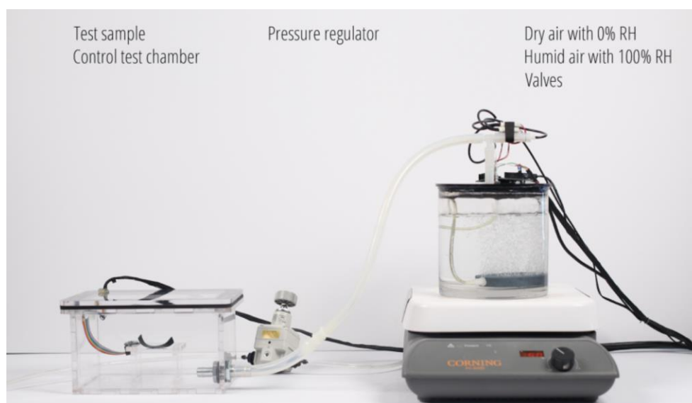
fig. S3. Customized humidity-controlled chamber. The setup include three main parts: The first module is the digital humidity sensor that is contained within the humidity control box. The second module is the controlled air source. There are two air streams that contain 0% RH and 100% RH respectively. The third module is the interface and control module. Through the computer interface, users can input desired RH for the test chambers. It takes between 20 seconds to 1 minute for the system to react and reach the desired RH. The equipped digital humidity sensor (HTU21D(F), Adafruit) has a
