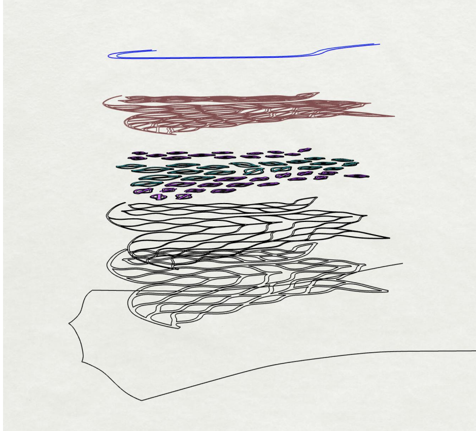
fig. S9. Assembly of a female running suit focused on the back ventilation through heat press. Layers from the top to the bottom (from the layer that is the closest to the skin) are mesh fabric for spacing, thermoplastic polyurethane (TPU) for bonding with applied heat, stretchy fabric, TPU for bonding, functional bio-flaps, TPU for bonding, and stretchy fabric as the main back panel.
