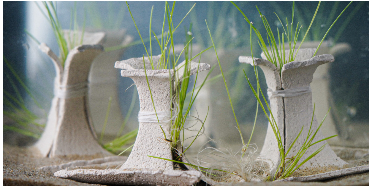
Figure 31. Before building large scale prototypes, we designed smaller prototypes of the form design to test design details such as increasing tile overlap and stability.
