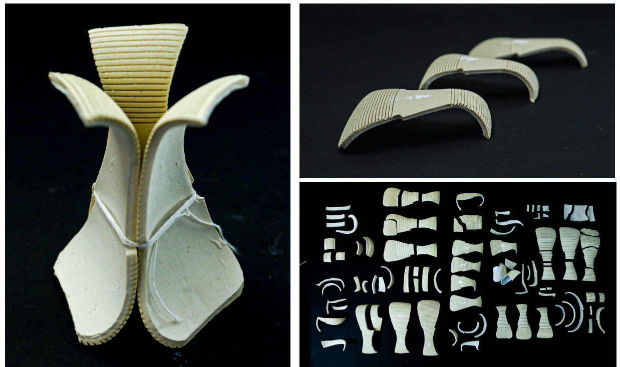
Figure 29. Ceramic samples used to chart the relationship between the grooving and the morphing.
