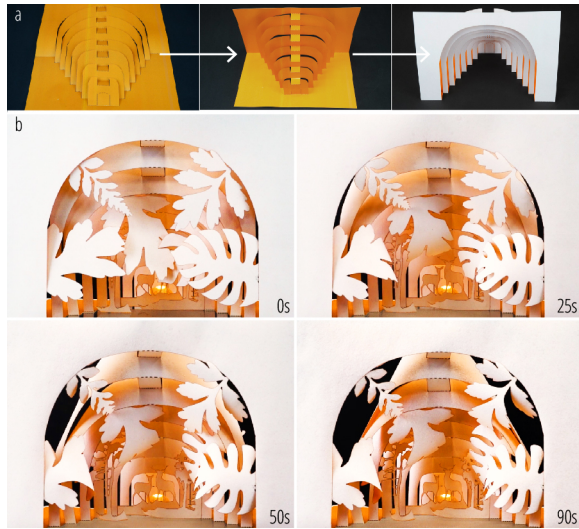
Figure 19: (a) Fabrication process - origami to fold into the shade in different depth and distance; (b) Different regions in the lampshade bend in sequences with time tags.
