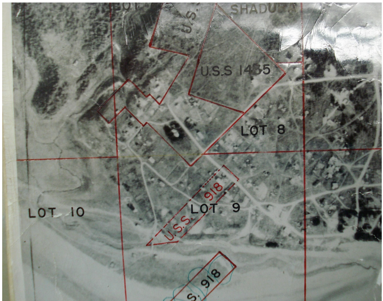
Aerial image of Kenai, 1949, overlain by surveyors' marks showing preexisting private land. This was used to prepare for the survey of old town home lots. Bureau of Land Management image via the National Archives.
