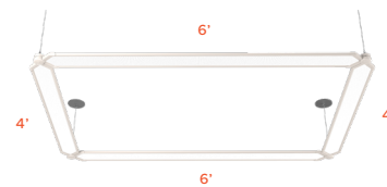
FSR (Square or Rectangle) pattern is fixed at 90°. FSR pattern shown with four fixed 90° arms.
