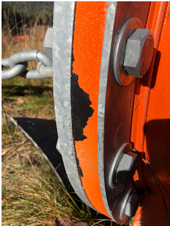
TPU Flame coating application error
