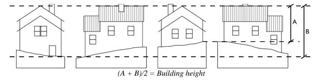
Building height of an accessory dwelling unit is measured from the average level of the highest and lowest point of that portion of the ground covered by the footprint of the accessory dwelling
