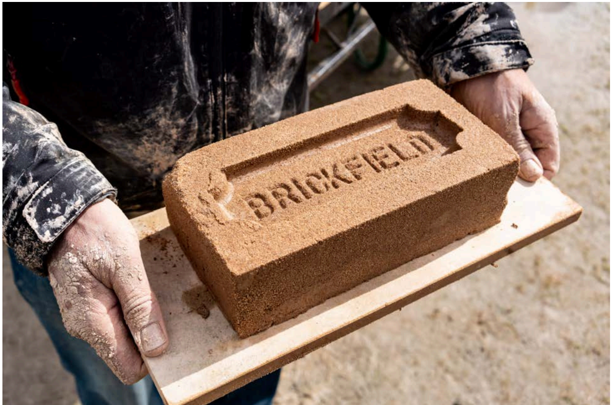
Handmade Brickfield brick using waste materials from the china clay industry Image credit: James Darling
