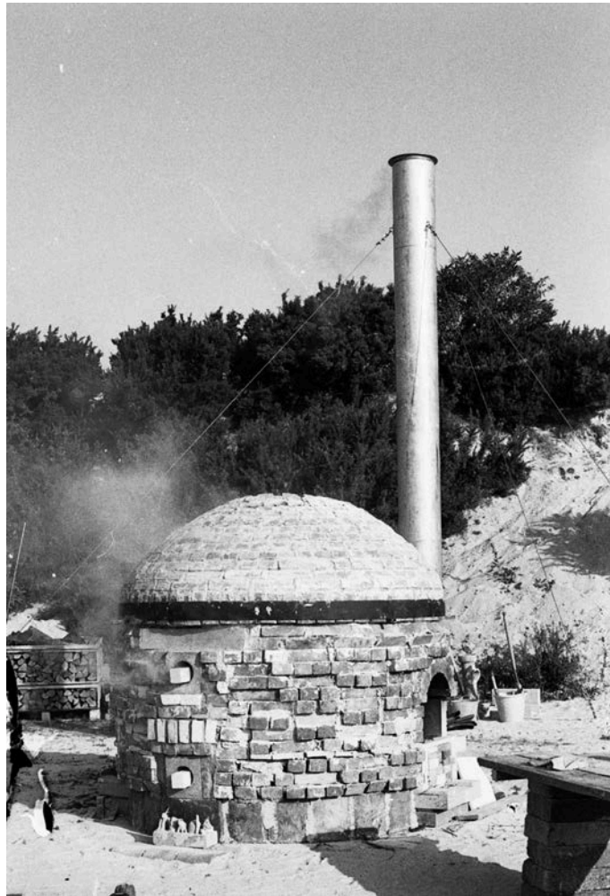
Brickfield mini-beehive kiln made using reclaimed bricks Image credit: Georgia Haseldine
