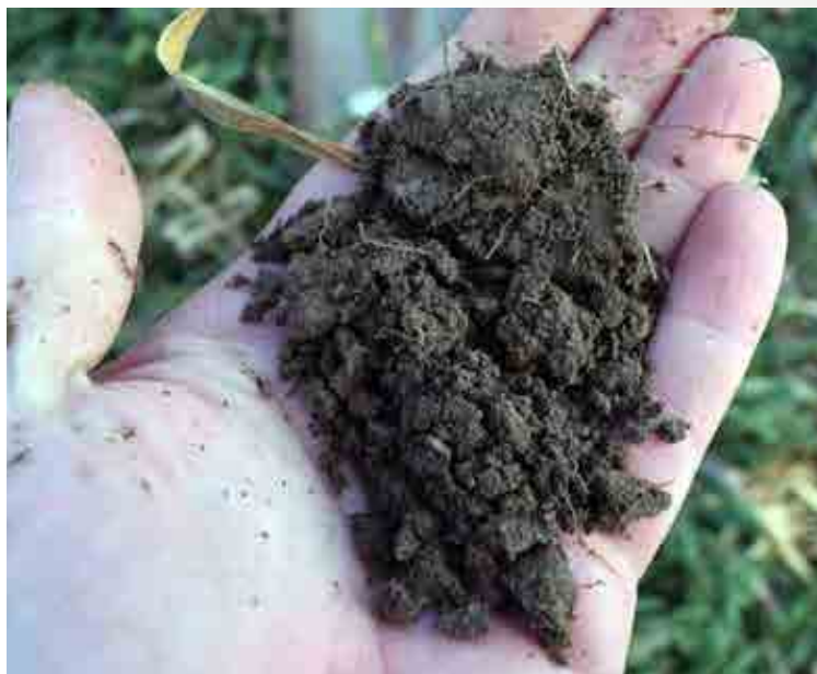
A good soil looks like black cottage cheese. It displays distinct aggregate structure, presence of roots, porosity for water absorption, and a dark color indicating the presence of carbon.
