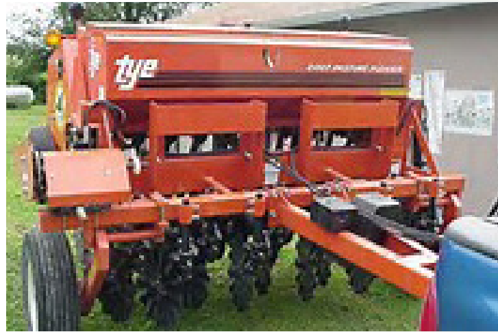
6 foot no-till fully mounted drill. Minimum of 40 horsepower required.
