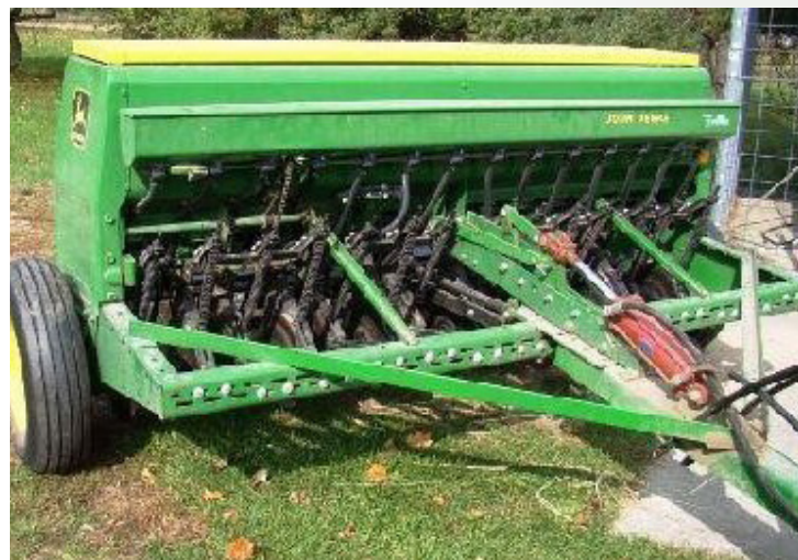
Small grain drill can be used to plant grass and legume mixtures.
