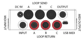
The white jacks on the rear panel serve as input and output connections. Plug your instrument into the white jack nearest to the power jack, and plug your amplifier into the white jack next to the USB port.
