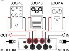
Connect your pedals as shown in the diagram above. Make sure to **engage** all of your pedals in the loops! The DPC.micro can bypass and engage them remotely only if the pedals are powered on and engaged.
