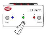
Tap the footswitches to engage or bypass each loop.
