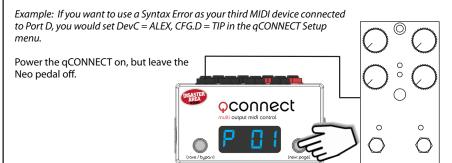
Hold and release the right footswitch on the qCONNECT until the device mode that you want to use is showing.
