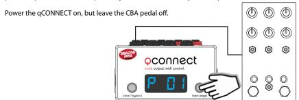
Hold and release the right footswitch on the qCONNECT until the device mode that you want to use is showing. We usually recommend that the device order match the order that the pedals are placed in your chain, so for example Brothers might be A, Warped Vinyl would be B, and Dark World would be C.
