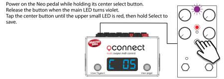
Power the Neo pedal off and back on, again holding the center button until the upper LED turns violet.
