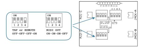
If you are using your SMARTClock to send taps or as a Favorite switch with the EXP port on Strymon pedals:
