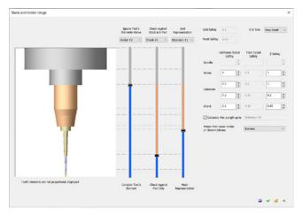
A new shank and holder dialog enables better user control and full transparent information over the different cutter assembly components including shank, extension, and holder stages, for considering or ignoring, for safety and for minimal clear length with complete feedback interactively
