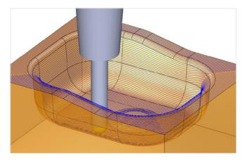
A start-to-end 3D Step Geodesic 3-axis toolpath on a steel cavity, with no re-entries, to achieve best surface quality without approach retract marks.
