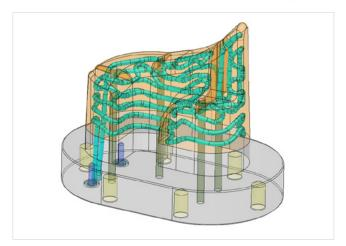
Automatically generated Conformal Cooling channel
