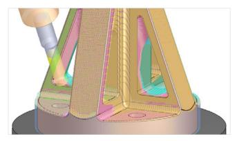
A Fixture rough cut, using automatic Rough 3 +2 axis set of operations. The stock is colored by the orientation. The directions are defined automatically by the system
