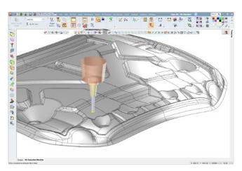
Finishing this car engine hood die tool using a Circle Segment cutter diameter 20mm, machining time can be reduces by 10% from 132 hours down to 119 hours compared to using A ball tool diameter
