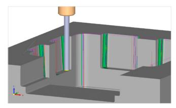
An efficient re-rouging at corners is done with the new "Corner Plunging" procedure, where the stock is removed by down cutting operations, including an option for forward steps.
