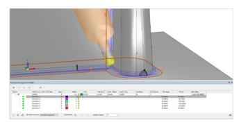
Zoom-in picture of a cleanup corner, machined in an inclined 3 + 2 axis orientation. The orientation was calculated automatically by the system, as part of the Guided Cleanup Auto Tilt function.
