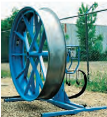
50" (1,270 mm) diameter capstan on Remote Mounting Stand.
