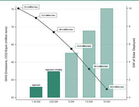
*Note.* This figure displays the emissions reductions of OPSB-approved solar projects, approved + pending projects, and hypothetical deployment scenarios summing to 5, 7.5, and 10 GW. Baseline emissions are calculated using 2018 Ohio eGRID data, <sup>3</sup> and removing the J.M. Stuart and Killen Stations, as well as the Conesville Plant, all of which are no longer operational. The mitigation calculation assumes a solar energy capacity factor of 25.2%, per NREL.
