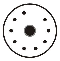
Do not insert tubes with missing or damaged pins. Do not insert the EL84 into a 12AX7 socket or vice-versa. See the Chassis Diagram or Tube Chart for the correct tube placement.
