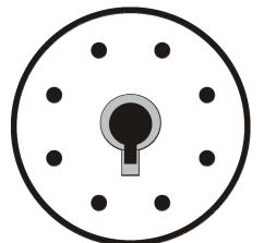
Do not insert power tubes with missing or damaged keys or pins.
