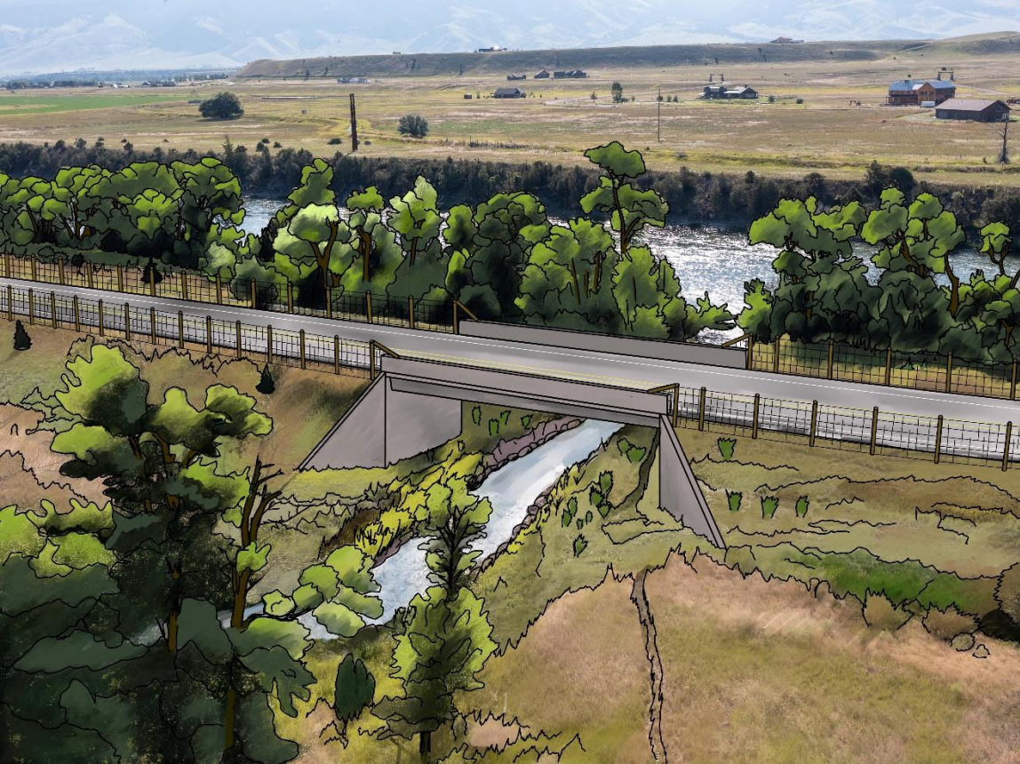
Figure 44. Existing roadway and culvert and conceptual rendering of upsized underpass in the Mill Creek Priority Site
