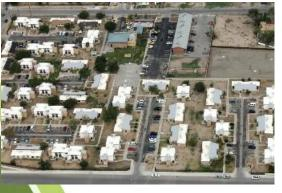
he days of black tar and asphalt roofing materials may be coming to an end. White polyvinyl membrane roofing material is growing in popularity because of its durability and energy efficiency. Because this material reflects the heat of the sun and provides decades of performance, it meets Energy Star sustainability standards and can qualify a property for Leadership in Energy and Environmental Design (better known as LEED) certification by the U.S. Green Building Council.
