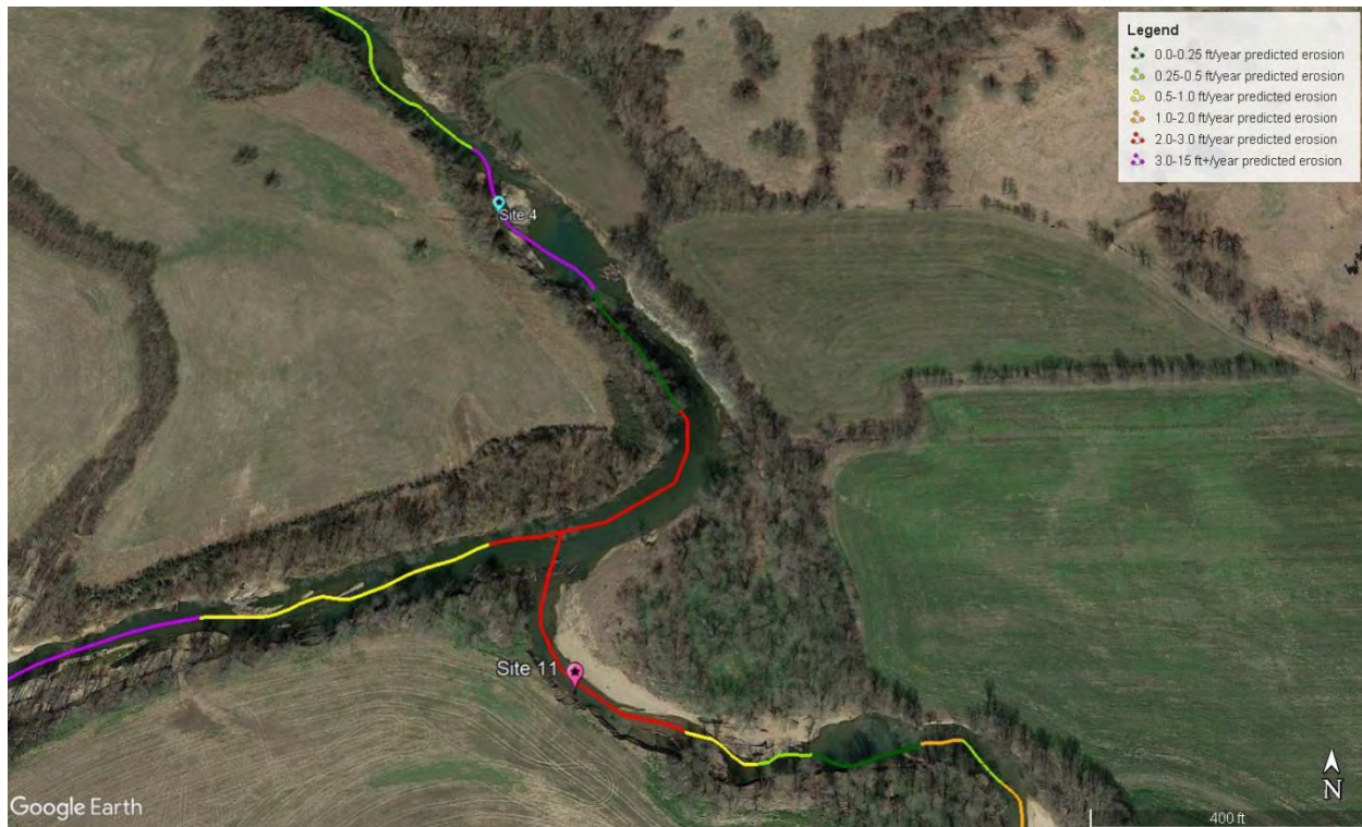
Figure 1. 2016 overview of study sites 4 & 11. Based on the best available information at that time, erosion predictions were made for each stream bank line segment and color-coded (see Legend).
