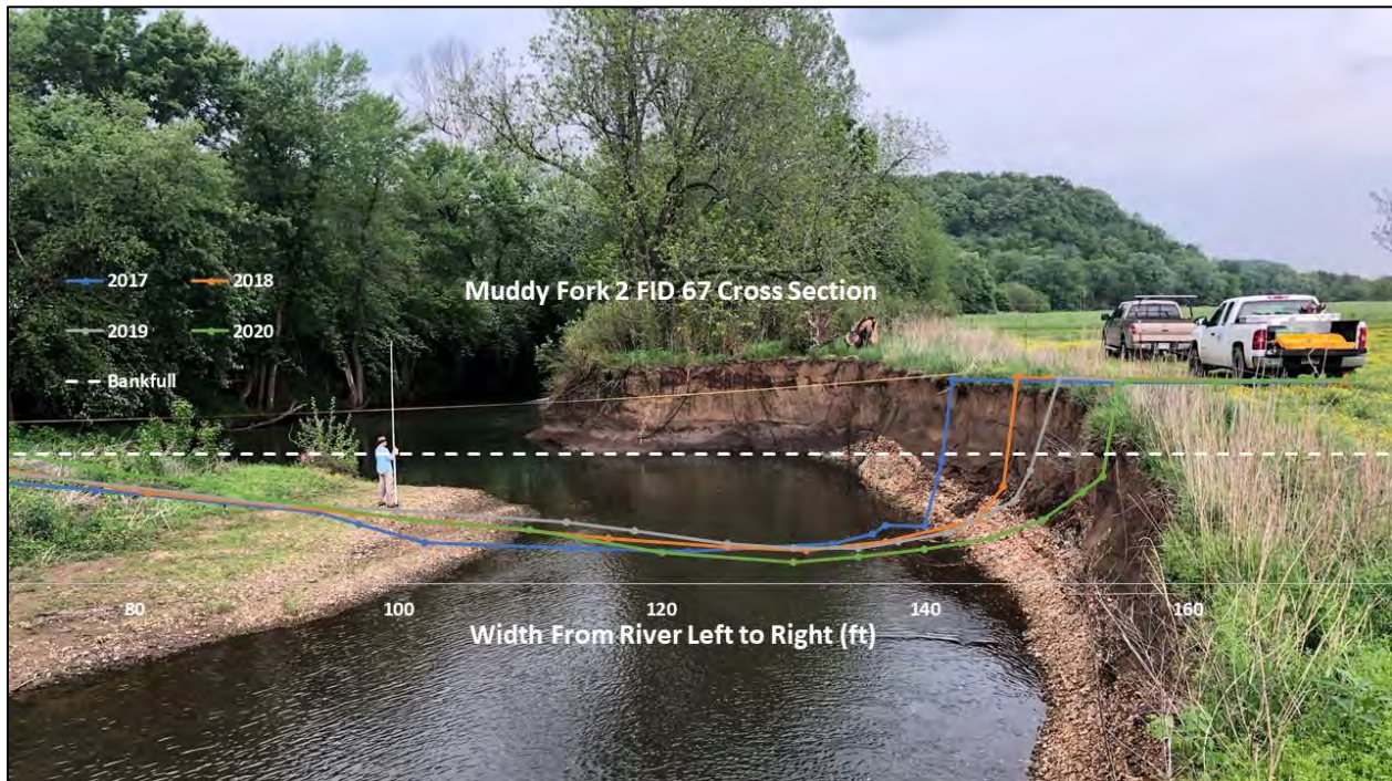
Figure 3. 2017-2020 Cross section graph and 2019 data collection photograph overlay at survey site 2.
