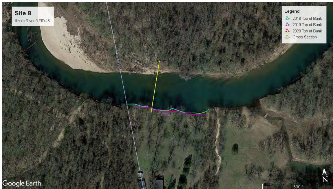
Figure 26. Planform view of Illinois River 3 FID 46 annual survey site. Illinois River flows generally East to West at this location. The light blue line represents the location of the study bank in 2018, while the purple line and red lines depict the top of bank location on the survey dates in 2019 and 2020 respectively. Google Earth Imagery Date: 3/4/2020.
