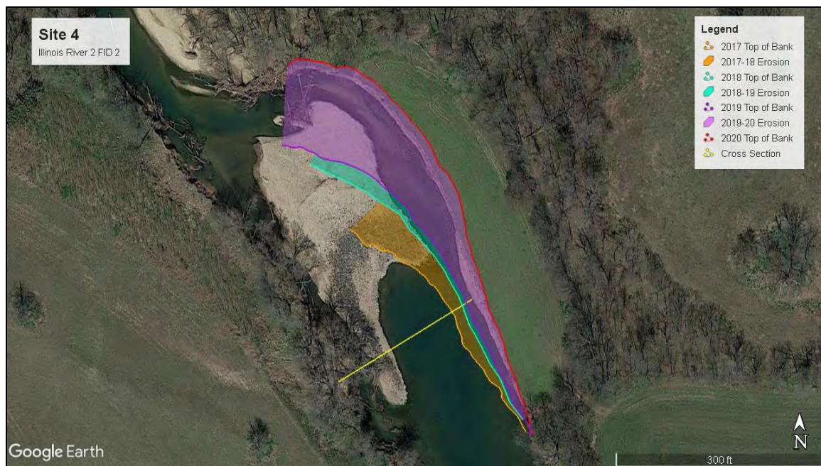
Figure 14. Planform view of Illinois River 2 FID 2 annual survey site. The river flows generally South to North at this location. The orange shaded area represents the bank/pasture lost to erosion from 2017-2018. The light blue shaded area represents widening of the river channel and land washed away from 2018-2019, while the purple shaded area depicts the river channel continuing to widen and a large area of eroded soil and grass that washed downstream from 2019-2020. Google Earth Imagery Date: 3/4/2020.
