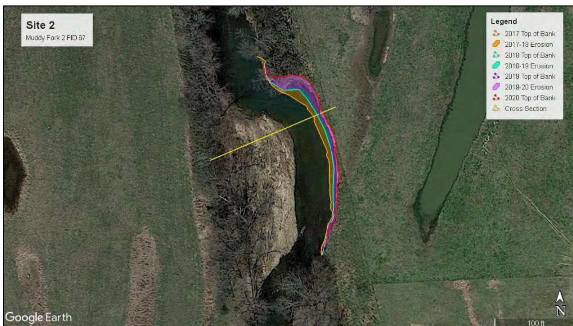
Figure 8. Planform view of Muddy Fork 2 FID 67 annual survey site. The creek flows generally South to North at this location. The orange shaded area represents the bank lost to erosion from 2017-2018, while the small light blue shaded area represents bank lost from 2018-2019, and the purple shaded area depicts land eroded from 2019-2020. Google Earth Imagery Date: 3/4/2020.
