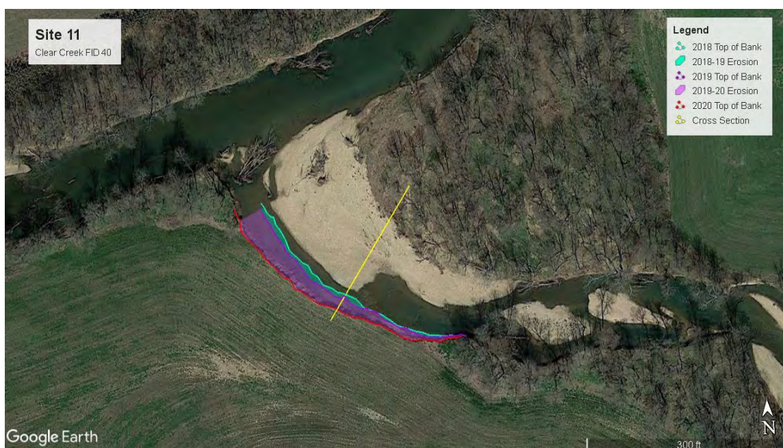
Figure 35. Planform view of Clear Creek FID 40 annual survey site. Clear Creek flows in from east to west and confluences with the Illinois River immediately downstream of the study bank. The area shaded in light blue represents stream bank erosion that took place on Clear Creek from 2018-2019, while the area shaded in purple depicts erosion that occurred from 2019-2020. Google Earth Imagery Date: 3/4/2020.
