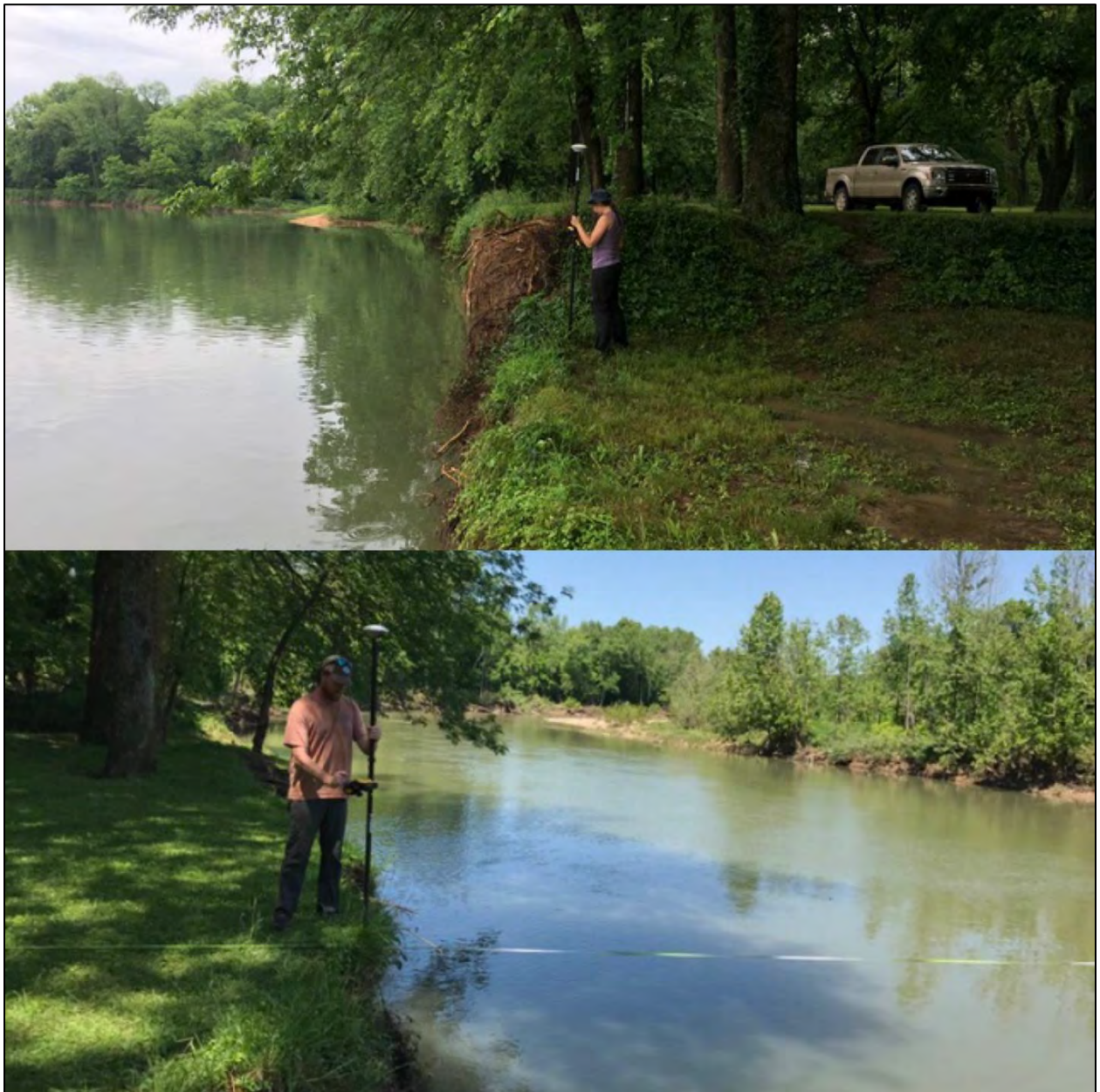
Illinois River 3, FID 46, 2018 (top) & 2019 (bottom), GPS marking of current top of bank position.
