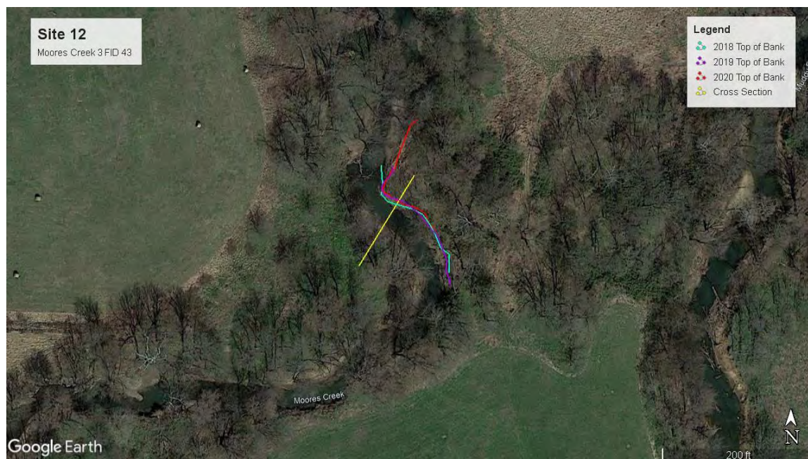
Figure 38. Planform view of Moores 3 Creek FID 43 annual survey site. The light blue line represents the location of the study bank in 2018. The purple line depicts the top of bank location on the survey date in 2019, and the red line represents top of bank in 2020. The annual top of bank lines appear to overlap at this scale, indicating that the bank has not moved tremendously through the 2-year study period. Google Earth Imagery Date: 3/4/2020.
