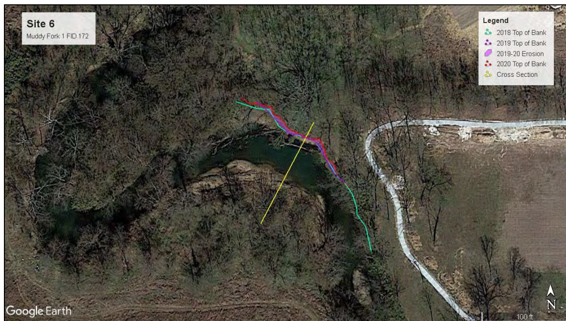
Figure 20. Planform view of Muddy Fork 1 FID 172 annual survey site. The light blue line indicates the target top of bank location in 2018. The purple line indicates the bank location in 2019, and the red line indicate the location of the top of bank during the most recent survey in 2020. Of note is that this area is experiencing rapid development in or very close to the active floodplain and riparian corridor of Muddy Fork. A paved trail that was not here in 2019 is clearly visible on this aerial as well as new building pads directly to the north of that trail. Google Earth Imagery Date: 3/4/2020.
