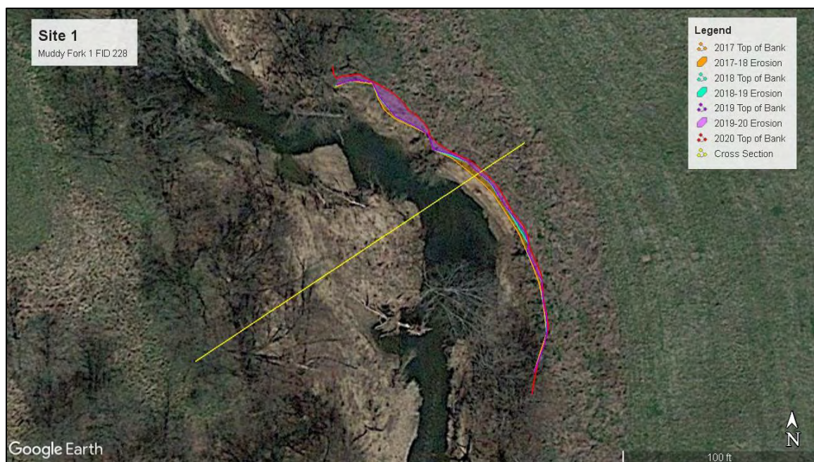
Figure 5. Planform view of the Muddy Fork 1 FID 228 annual survey site. The Creek flows generally South to North at this location. The small orange shaded area represents the bank lost to erosion from 2017-2018, while the light blue shaded area represents bank lost from 2018-2019, and the purple shaded area depicts land that washed downriver from 2019-2020. Google Earth Imagery Date: 3/4/2020.
