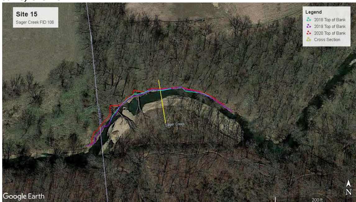
Figure 47. Planform view of Sager Creek FID 106 annual survey site. The light blue line indicates the top of bank location during the 2018 survey. The purple line illustrates the location of the bank in 2019, and the red line indicates the most recent top of bank location from the 2020 survey. Note that several large trees have recently fallen into the channel. More significant erosion is likely to occur here as a result of this disturbance. Google Earth Imagery Date 3/4/2020.
