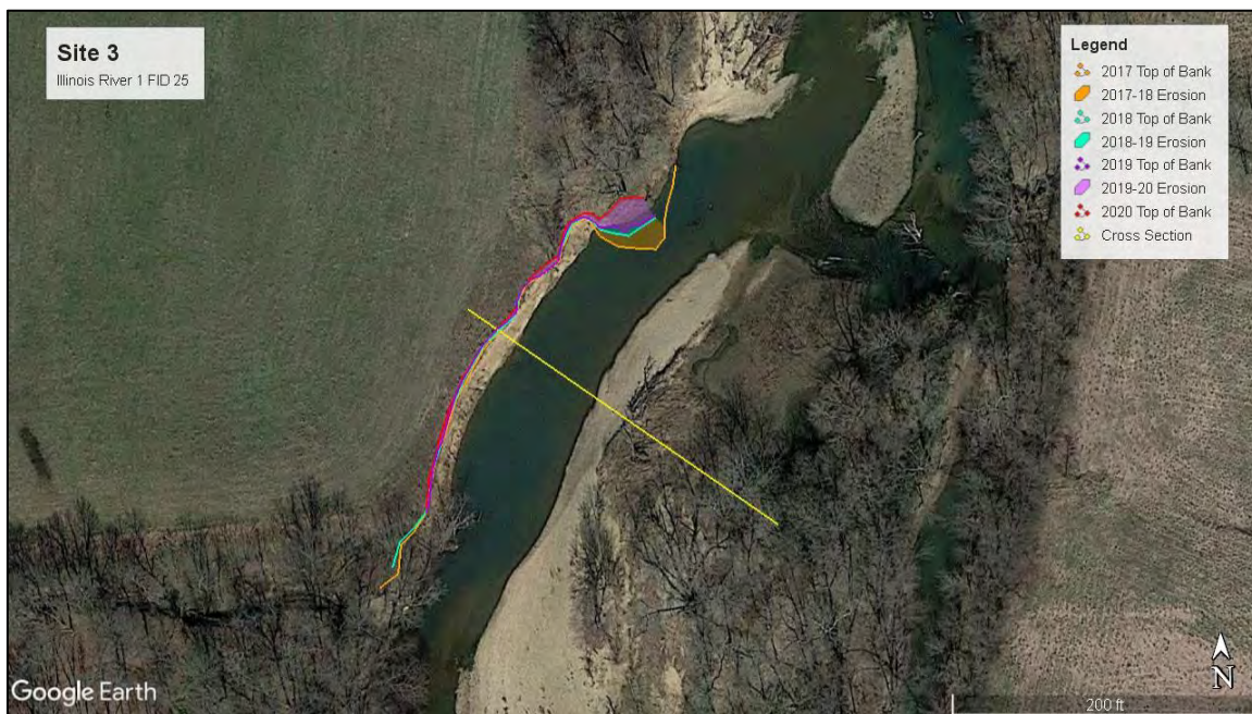
Figure 11. Planform view of Illinois River 1 FID 25 Permanent Survey Site. The orange shaded area represents bank lost to erosion from 2017-2018. The small light blue shaded area represents bank erosion from 2018-2019, and the purple shaded area depicts land lost to erosion from 2019-2020. Google Earth Imagery Date 3/4/2020).
