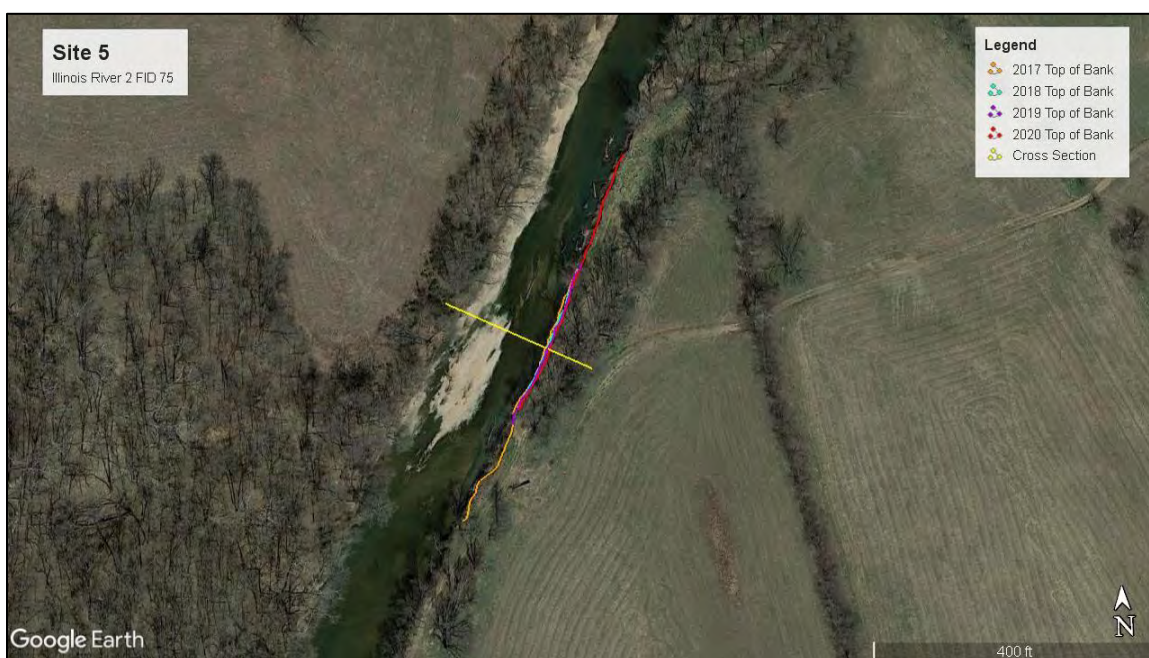
Figure 17. Planform view of Illinois River 2 FID 75 annual survey site. The river flows generally South to North at this location. The orange line represents the location of the study bank in 2017. 2018 is represented as a light blue line. The purple line depicts the top of bank location on the survey date in 2019, and the red line represents top of bank in 2020. All of the lines overlap slightly, indicating that the location of the top of bank has not moved tremendously through the 3-year study period. Google Earth Imagery Date: 3/4/2020.
