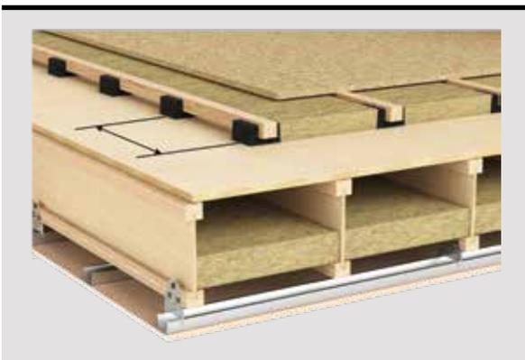
**Figure 5: QB Quiet Batten™ Spacing**
