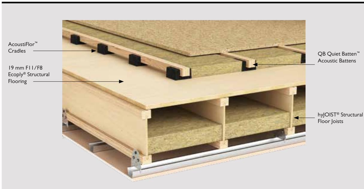
This acoustic system can be applied for use in applications including most domestic and commercial buildings including residential apartments and offices where live loading does not exceed 4.0 kPa and/or 2.7 kN. Where live loading exceeds these parameters Specific Engineering Design (SED) is required.
