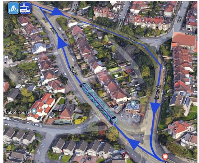
At the Bath Rd/Eagle Rd junction the double track would split into a single track running south on Bath Rd and a single track running north along Eagle Rd.
