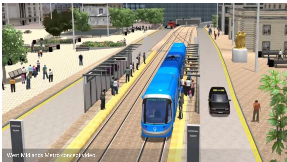
Fig. 11 - central reservation tram stop with pedestrian controlled traffic lights
