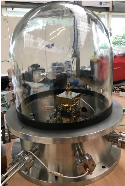
Figure 6: Bell Jar Vacuum Chamber Setup Testing Comet-1000
