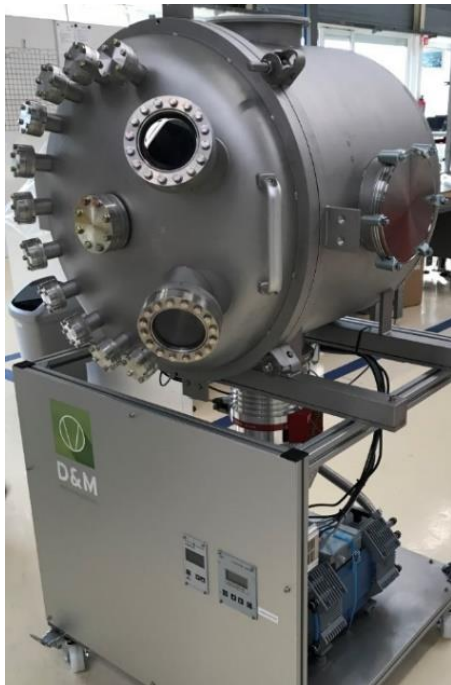
Figure 7: Functional Test Setup Suitable for Comet-8000 (Vacuum Chamber 700 mm diameter x 700 mm long)
