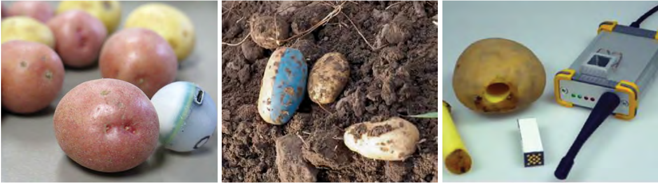
Figure 5. Devices for measuring impacts during potato harvest and packing: From left the Series 500 IRD (Techmark, USA), TuberLog (Esys, Germany) and Mikras (Esys, Germany)
