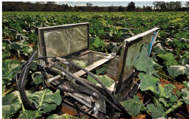
Figure 3. Measuring nitrous oxide emissions in a broccoli crop; nitrous oxide is an extremely potent greenhouse gas
