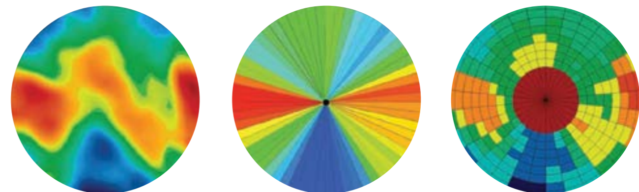
Figure 4. The data graph (left) based on EM soil mapping and soil moisture probe data; sector graph (centre), which adjusts the pivot speed to provide more or less irrigation, concentrating on the outer portions of the cropping area; zone graph (right) which further divides the area into concentric rings, allowing precise irrigation of each area (Images from Reinke www.reinke.com).
