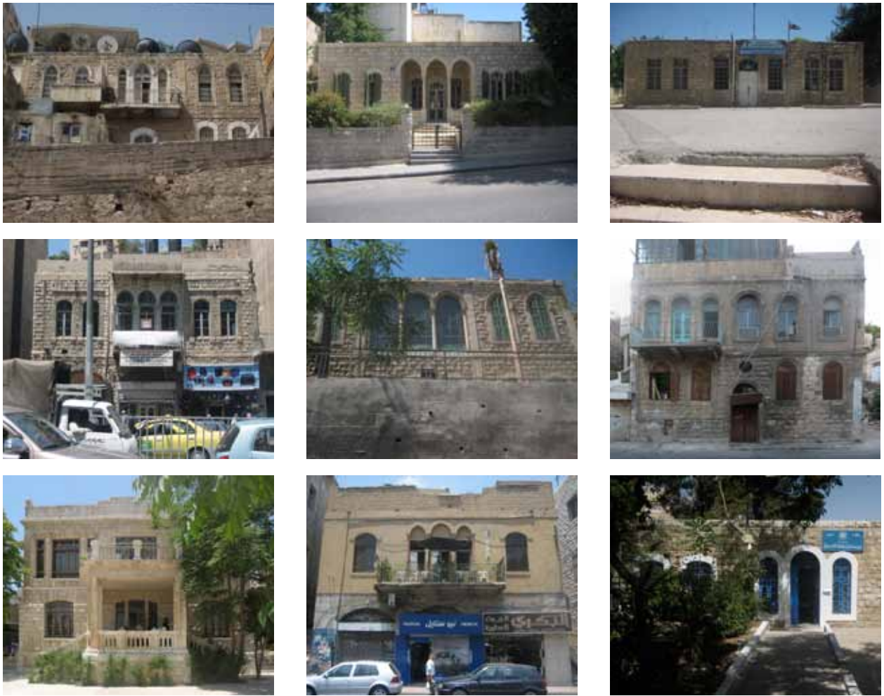
Fig. 3.12. Tripartite masonry opening ensembles are perhaps the most characteristic exterior architectural detail of typical villas and commercial structures built in Amman during the mandate period.
