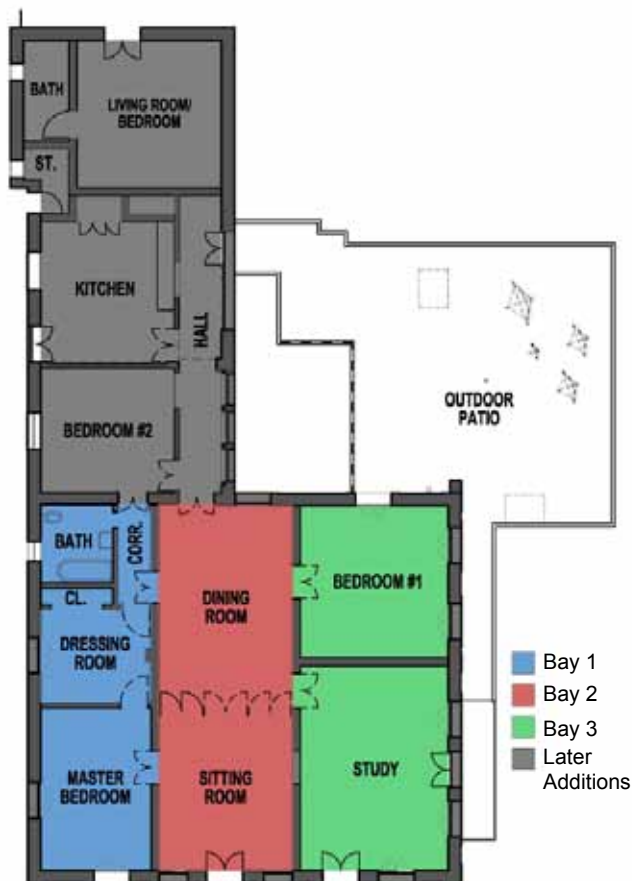
Fig.2.9. (Above) Speculated original floor plan showing three aisle design. (Left) Current layout as of July 2009 showing later alterations. Fig. 2.10. (Below) Decorative floor tile in central hall.
