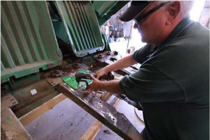
Drill the two rear holes (nearest to the hinge points) with a 3/8" diameter drill. A mag-based drill works the best for this operation.
