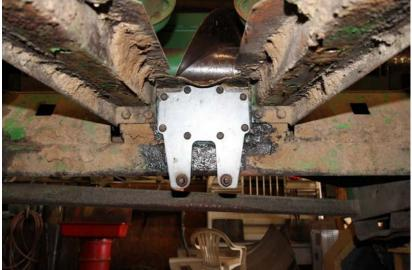
Clean rust and scale off the top of the deck plates to prepare for drill work and installation.
