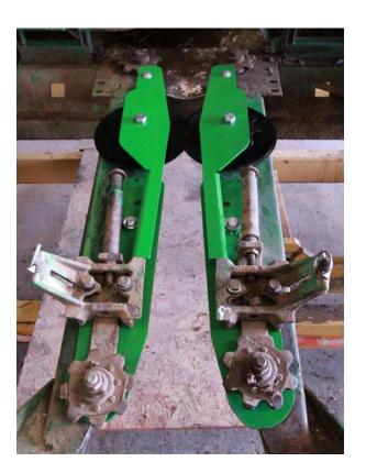
Install gathering chains noting that the "lugs" must be staggered evenly, and tighten pre-load springs per the combine header service manual specifications, approximately 1/8" to 1/4" gap at the adjusting bolt head.
