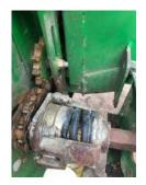
Remove the inboard PTO shaft cover to expose the steel shaft, that will help you pull the hex shaft out of the outboard assembly
