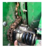
When re-installing hex shaft, make sure inboard auger drive chain does not rub on bottom below the tensioner
