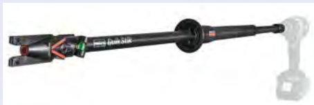
Figure 4-30. Simpson makes the Quik Stik to facilitate drilling the SDWC. It sells for under $200 and holds the structural screw at the proper drill angle. This tool is useful for new construction and may eliminate the need for pre-drilling in retrofit applications, especially for softer siding. For hard siding, some pre-drilling may still be required. An impact driver is hooked up on one end and the SDWC loaded on the other (see Reference Link 45).
