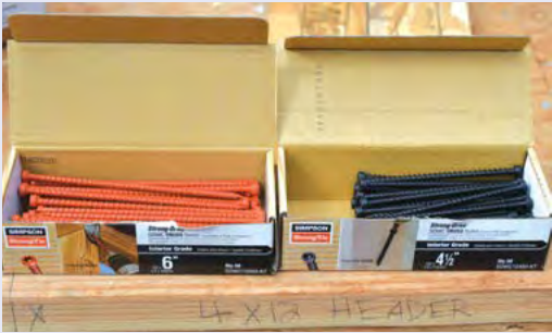
Figure 4-20. SDWC Structural Screws at a new construction job site on O’ahu. Their use was approved by the building department, building inspectors, and the project structural engineer to meet current building codes. The screws can also be used as a retrofit on existing double-wall houses as shown in this demonstration. The 6” orange SDWC screw can tie the truss to the double-top plate and the double-top plate to the stud (Connections A and B) in Figure 4-19. The 4.5” black SDWC screw can be used to tie the stud to the single-sill plate (Connection D).
