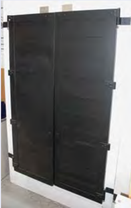
Figure 4-37. Colonial shutters are typically made of aluminum or fiberglass. During a storm, the panels are closed and secured along the vertical center of the window. During good weather, the panels open along hinges on the side of the window and rest flat against the wall in a decorative manner. Photo courtesy of Hurricane Secure.
