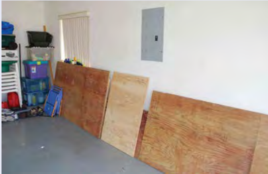
Figure 4-56. Once the panels are created, they can be stored in the garage and take up minimal space if stacked neatly along the side of the garage, with the smallest pieces closest to the wall. Panels should be checked each year for any warping or rotting and replaced as needed.
