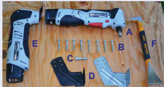
Figure 4-10. In the case where the molding needs to be removed, this can be easily done with a multi-tool (E) and a nail-trim remover (F).
