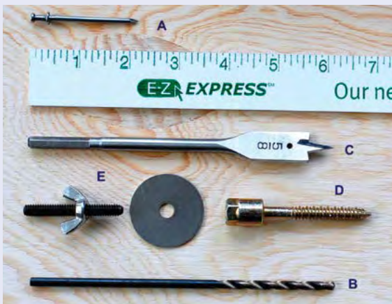
Figure 4-51. Many panels have permanent fastenings attached to the house. (i) After attaching the panel to the frame with two duplex nails (A); (ii) holes are drilled with the bit (B) into the panel and wood frame; (iii) then a spade wood boring bit (C) cuts wider holes into the panel and frame; (iv) a lag screw anchor with female receptor (D) is screwed into the wood frame; (v) and the panel is attached with washer and wing nut (E).
