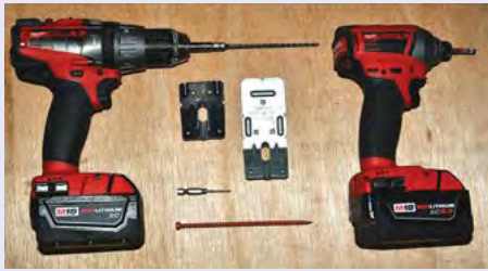
Figure 4-28. For most materials it is easy to drill the SDWC. Simpson provides a metal guide to hold the SDWC at 22°. Hardie Siding however is difficult to drill as the material is made of hard fiber cement. It may be necessary to pre-drill first with a short bit, and second with a longer, wider bit.
