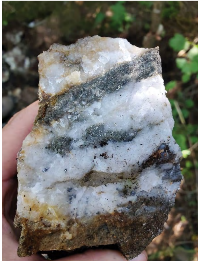
Photo 01 quartz vein from Sample 697925, assaying 7.02ppm Au, with minor pyrite and galena in sheared, silicified granodiorite containing 1-2% disseminated pyrite.
