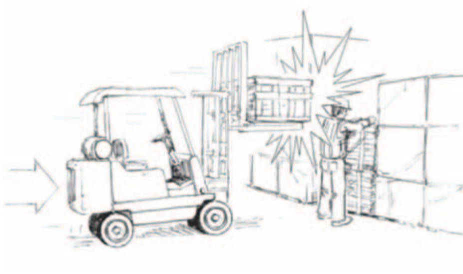
Worker crushed by forklift.
