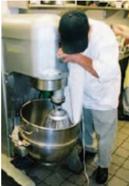
Apron caught in mixer with no guarding
