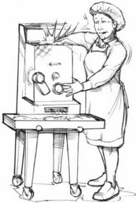
Wearing loose clothing. Sleeve caught in mixer and broke worker's arm.
