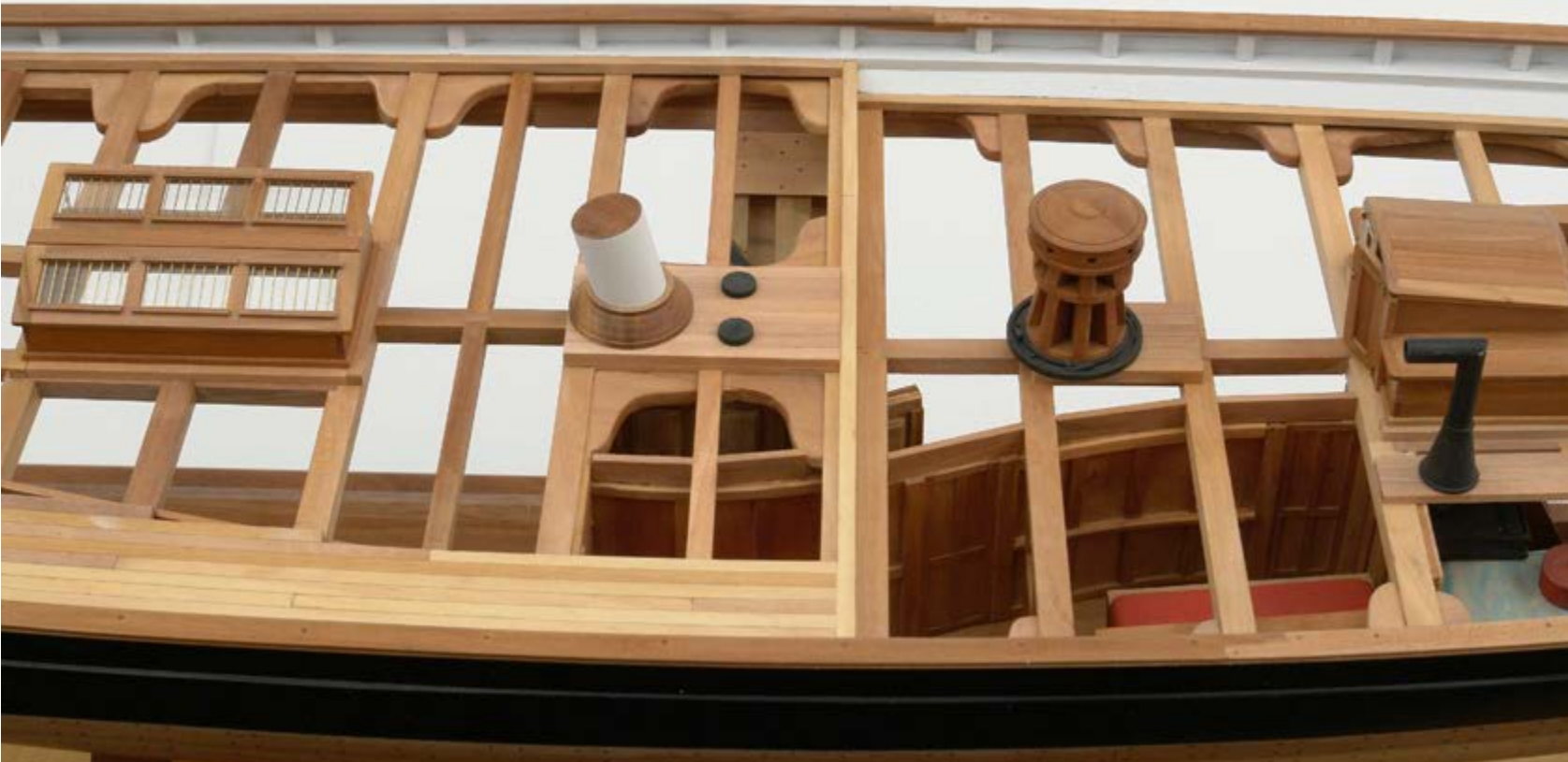
McCaffery's unique approach of only partially planking the deck allows us to look downward at the layout and fixtures below deck.
