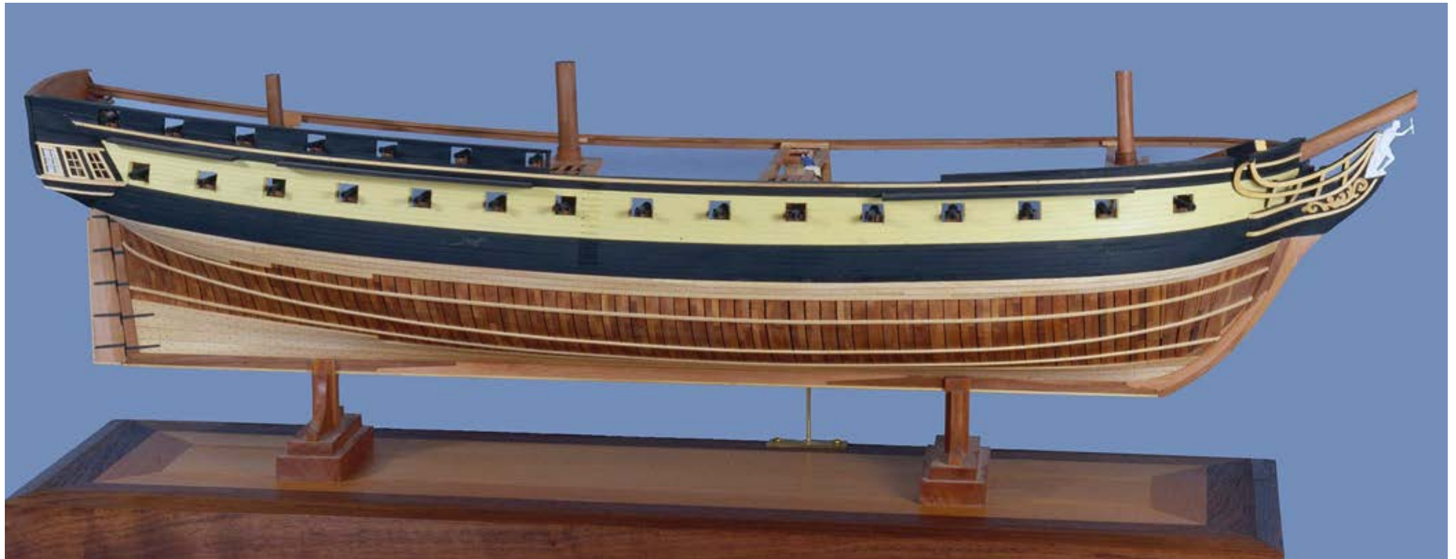
The starboard side of the model clearly shows the bulk of the massive hull. McCaffery has left most of the planking off to give us a clear view of the framing of the USS Constitution, painted in her original yellow ochre and black colors. The 1 1/2" Hercules Figurehead (shown above) measuring 12' on the actual vessel is carved from a single piece of boxwood and painted white.
