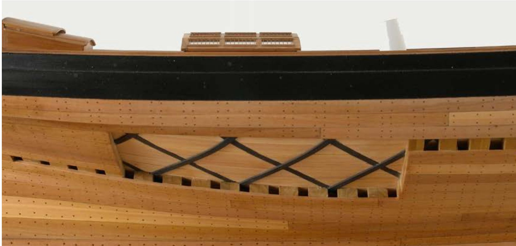
America was one of the first vessels to be built with the diagonal iron strapping seen above in McCaffery's model. This kept her hull from sagging or "hogging" over her long life.
